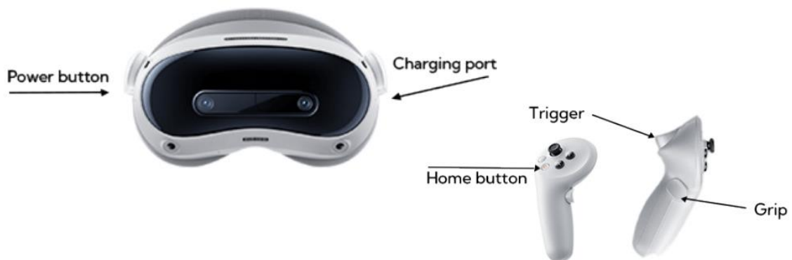
Figure 2. Control elements and interface layout of the Pico 4 Ultra system
