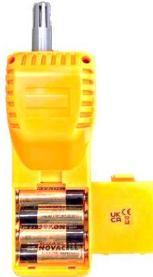
Figure 2. Installing the device power source - batteries
