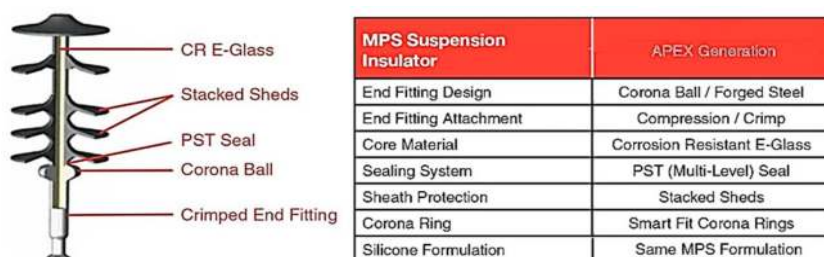
Figure 2 – Design of MPS Insulator [4]
